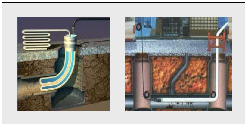
Figure 49 – Illustrations de la technique de chemisage
